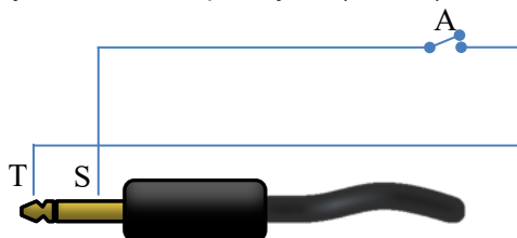
Layout 1, “mono” pin layout (default)
