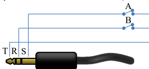
Layout 3, alternative, “mono-like” tip common, pin layout
