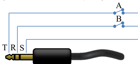
Layout 2, normal “stereo” pin layout
