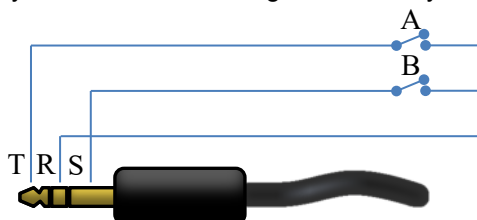
Layout 4, alternative, ring common, layout
