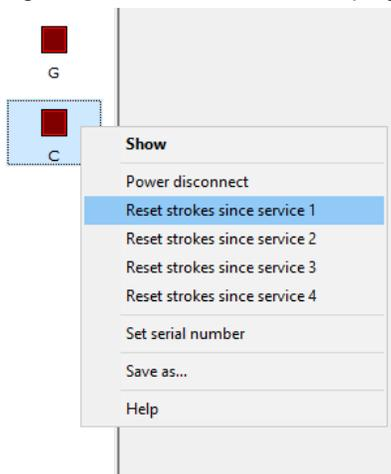
2. To reset the counter for channel X, select **Reset strokes since service X**.
