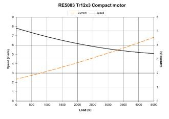
Charts show average figures for 24V actuator using stabilized power supply. All figures with ambient temperature of 20°C. Accuracy: ±5.
