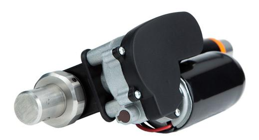
For an absolute feedback function, the actuator will be equipped with a multi turn precision potentiometer. In order to cope with the wide range of different stroke and pitch a gearbox is connected between the actuator motor output shaft and potentiometer shaft, the gear ratio is adapted to current stroke and pitch in order to have optimal feedback resolution for the application.
