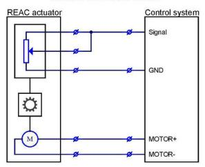
Signal connected to VCC via internal pull-up resistor. Less cabling but decreased accuracy.
