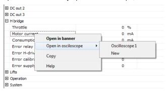
Up to four values can be shown in one oscilloscope tool.
