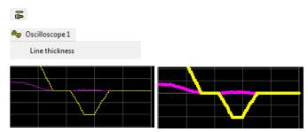
To the left at the bottom of the black area the scaling, along the X-axis is shown. Usually it is time based. And when time based it is indirectly derived from then time set in the tools lower toolbar.
