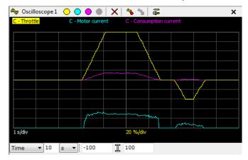
In this example the oscilloscope channel which shows Throttle is selected. This can be determined by looking at which one of the text labels at the top of the black area is reversed. It can also be determined by looking at the tools menu, where the currently selected one will have a checkbox.
