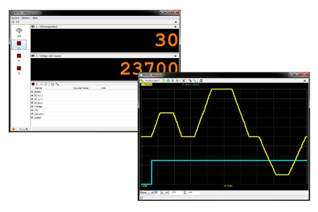
REAC Service Tool is a PC software for maintenance of products in our RCS series. The tool can be used to control customizable settings, perform common service tasks, and to monitor system behavior. Engineers might find it useful when evaluating application solutions. Service technicians can use the tool for regular maintenance tasks as well as for troubleshooting.
